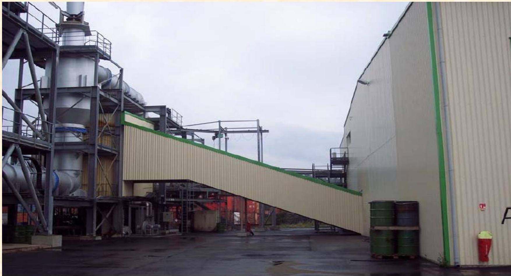
Photo Nr.6 Covered conveyer Shredded waste is delivered to the reactor filling hopper.
