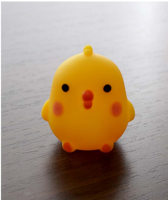
Photo 3 KE-PVC-toy-09 with highest level of DnOP (Di-n-octyl phthalate).
