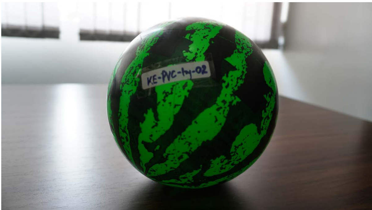
Photo 5 KE-PVC-toy-02 with highest level of both SCCPs and MCCPs.
