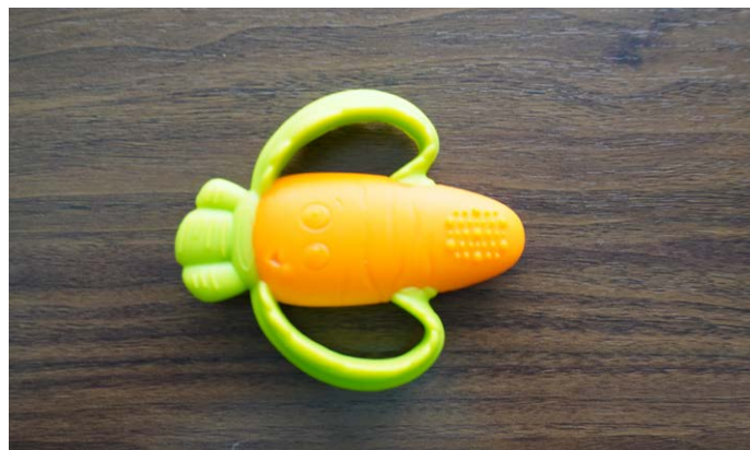
Photo 4 The KE-PVC-toy-06 teething toy is of concern, as it contains the second-highest level of UV-326.
