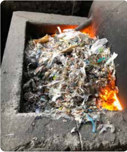
Figure 9. Plastic used as fuel to create steam. Photo: Ecoton
