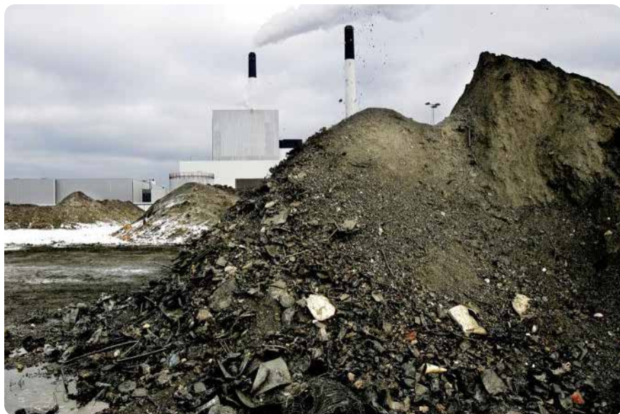
Figure 1: Waste incinerator in Copenhagen with pile of bottom ash; Source: (Borking 2011). In many EU countries is bottom ash used for roads construction and pavement. In some cases it also includes fly ash.
