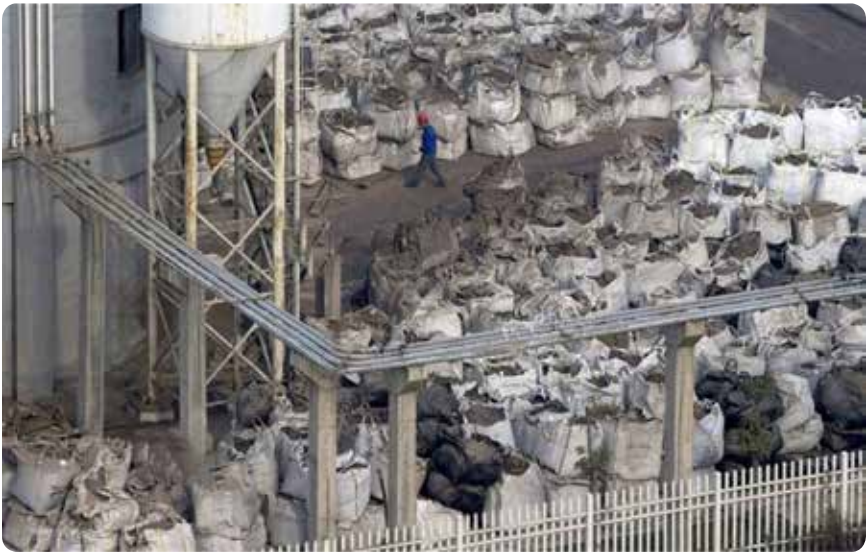
Figure 8: Fly ash in big bags stored exposed to the elements in MSW incinerator in Hanyang city, Wuhan, China. Source: (Zhang, Huang et al. 2015).
