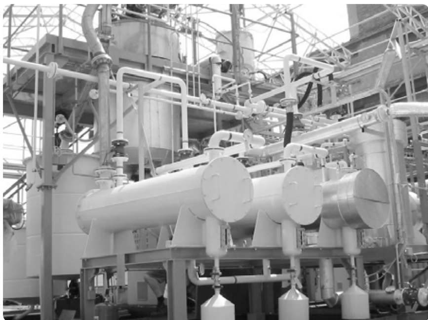
Figure 31: BCD destroyed POPs as second processing step in Spolana Neratovice, Czech Republic. Source: Kubal, Fairweather et al. (2004).
