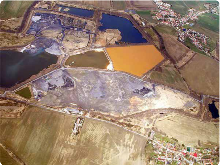
Figure 12: Aerial photo of the lagoons remaining after uranium ore reprocessing at a plant in Mydlovary, Southern Bohemia (Czech Republic). The lagoons are already partly filled with waste mixtures including fly ash. Source: mail.oakrupkovo.cz
