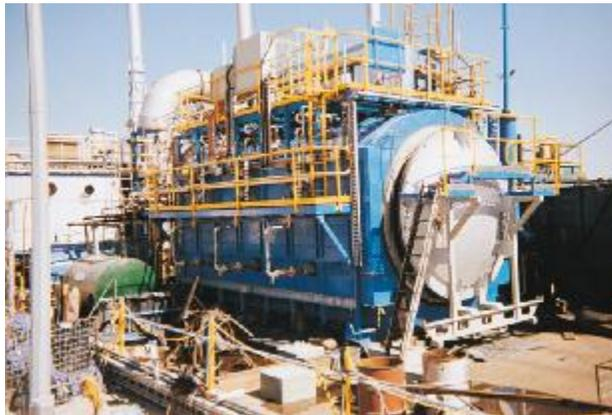
Liquid and solid wastes are placed into the TRBP, which is then heated to approximately 600°C in a hydrogen-rich (oxygen deficient) atmosphere. Contaminants that volatilize from the solids and liquids are then swept into the GPCR reactor for destruction.
