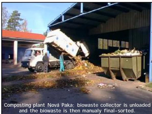
Composting plant Nová Paka; biowaste collector is unloaded and the biowaste is then manually final-sorted.
