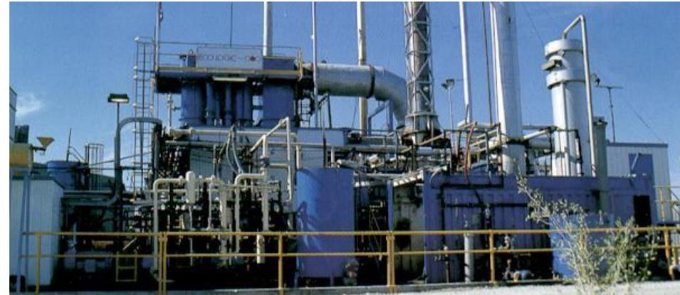
Volatilized contaminants from the TRBP are swept into the reactor, where GPCR occurs in a hydrogen-rich (oxygen deficient) atmosphere at approximately 875°C. Gases exiting the reactor (primarily methane, hydrogen and hydrogen chloride, are scrubbed to remove heat, particulate and acid, and then stored for reuse as a fuel.
