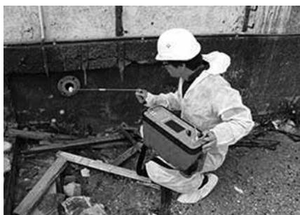
Figure 1: Example of a contaminated site investigator using a portable mercury vapor analyser.
